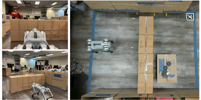
Fig. 1: The setup considered in PROBE involves a Go1 robot dog and obstacles that can potentially obstruct its path. Some planar obstacles, such as the long frontal box in the image, are movable, while others are fixed to the ground. A transformer network reconstructs the locations and sizes of the obstacles, including the occluded ones, from a history of proprioceptive data that the robot receives while exploring the scene without vision.
